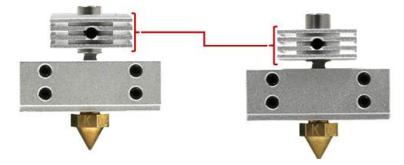
7. If you do not have a silicone sleeve, adjust the heat sink so that it is flush with the bottom of the large cylinder.
