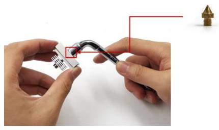
2. Insert a cleaning rod completely through the hotend and ensure that tube is completely clear of blockages.
