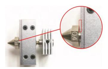
3. Hold the heating block, and tighten the throat tube by rotating the heat sink. Rotate until the nozzle "catches" on to the tube (begins to spin).
