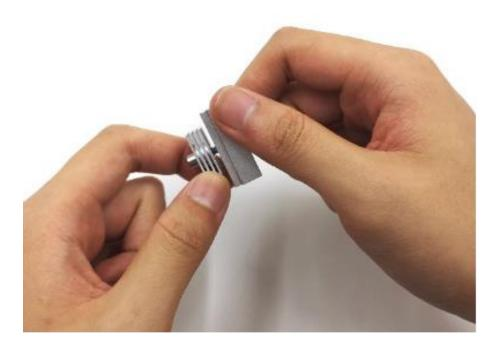
4. Hold the heating block, and tighten the nozzle completely with an 8mm socket wrench. Check that a gap between the nozzle and the heating block has been maintained.
