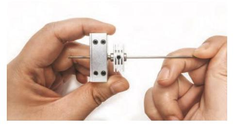
3. Install the new nozzle into the heating block. Do not tighten it completely. Ensure that there is a visible gap between the nozzle and the heating block.
