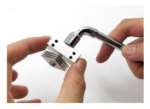
5. Re-attach the silicone sleeve, then loosen the retaining screw on the heat sink. Place the hot end assembly on a flat surface and rotate the heat sink so that the retaining screws face outward.
